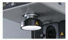
Example of attaching the LED circular illuminator on the PJ-Plus
