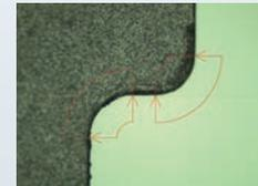
Measurement of micro radii is easy with the correct magnification
