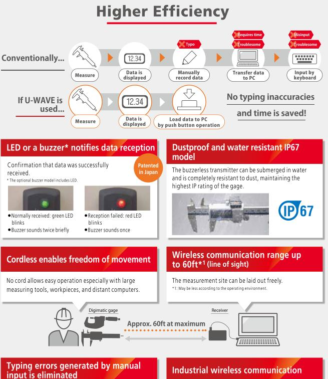
The measurement data can be transmitted directly by a single button operation.
