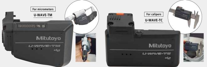
U-WAVE-TM for micrometers and U-WAVE-TC for calipers are available, both as the buzzer type and water/dust-proof IP67 type. The buzzer type notifies the normal reception of data by LED and buzzer sound. The water/dust-proof IP67 type is designed for a harsh environment and as such is only equipped with LED notification of data reception.
