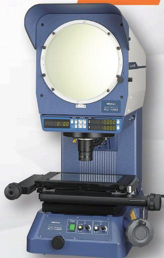
High accuracy profile projector with turret for use of multiple magnifications.
