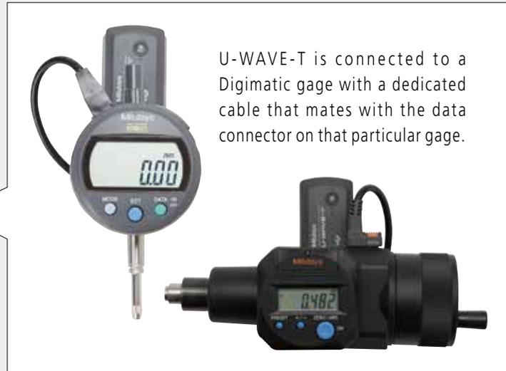
The buzzer type and water/dust-proof IP67 type are available. The buzzer type notifies the normal reception of data by LED and buzzer sound. The water/dust-proof IP67 type is designed for a harsh environment and as such is only equipped with LED notification of data reception.
