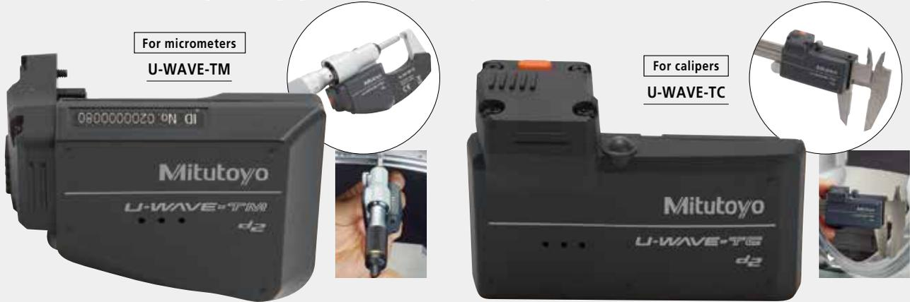
U-WAVE-TM for micrometers and U-WAVE-TC for calipers are available, both as the buzzer type and water/dust-proof IP67 type. The buzzer type notifies the normal reception of data by LED and buzzer sound. The water/dust-proof IP67 type is designed for a harsh environment and as such is only equipped with LED notification of data reception.
