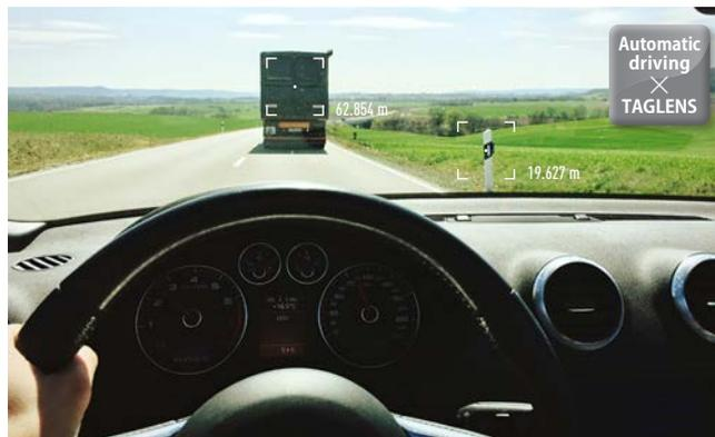
Use TAGLENS for automatic driving, so that all moving objects in front of the vehicle, such as cars and people, stay in focus, allowing reliable monitoring of the vehicle's intended path.
