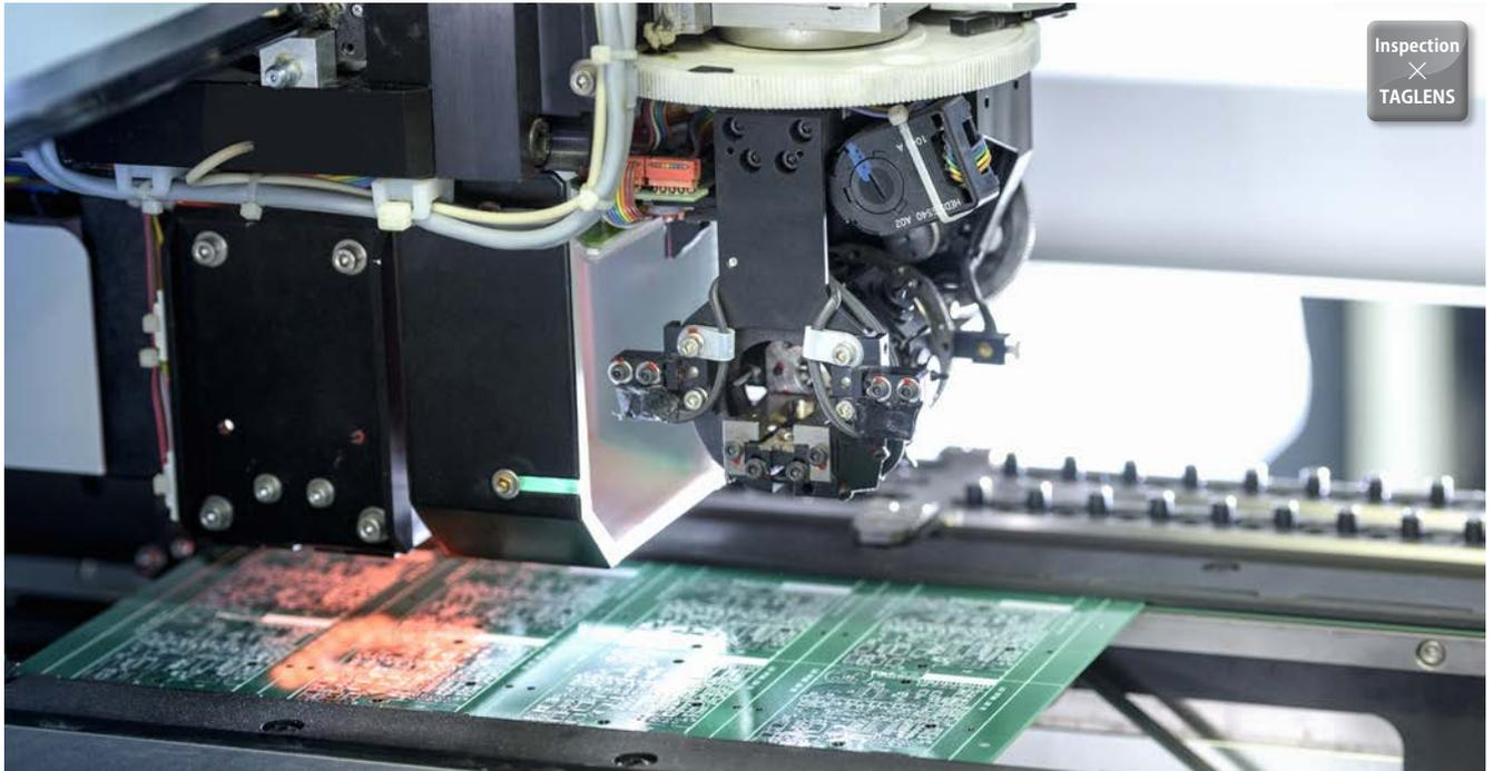
TAGLENS allows instantaneous, accurate checking of multiple subjects with different heights to be focused correctly, which have conventionally been checked by moving the camera vertically, since focal lengths differ.
