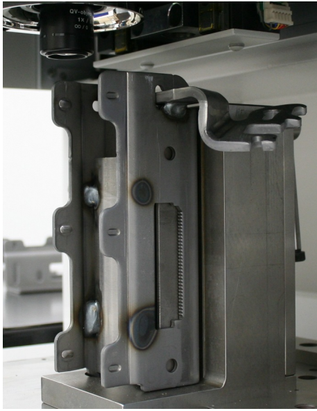
Fig. 1 Steering column bracket in assembled/welded state
