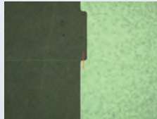
Measurement of the width of micro-recessed-forms cannot be accurately performed due to low magnification
