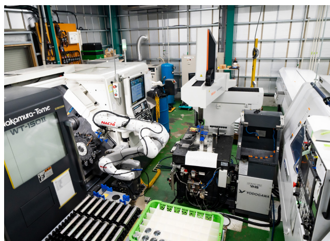
An automated production line comprised of two machine tools (left and right) and a measuring machine (center) taking advantage of the three-sided open structure
