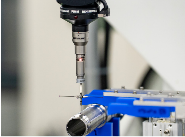
Inspecting a precision lathe machined part with the CMM
