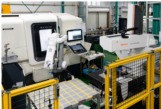
MiSTAR 555 installed at the production site together with machine tools and robots
