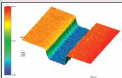
3-dimensional topographical result, data of micro-circuit
