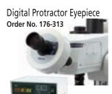
Magnification 10X, Field number 22 Resolution: 0.01°/1' Switchable Measuring range: 0-369.99° An angle is measured by simply rotating the cross hairs. Eliminates misreading errors that can occur with the scale type. \* Exclusive-use eyepiece is equipped (10X, Field number: 22)
