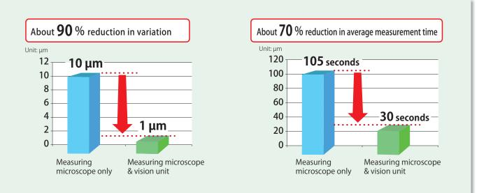
Measurement results and measurement times when measuring a width of about 20 mm thrice (continuous reciprocation) Measurement with the measuring microscope only
