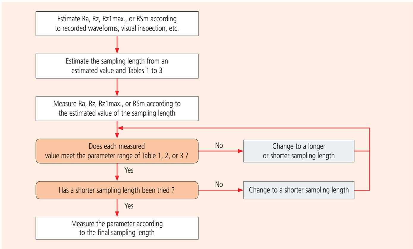
Fig.2 Procedure for determining the sampling length of a periodic profile if it is not specified.
