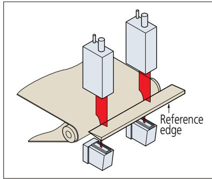
Measurement of spacing of IC chip leads
