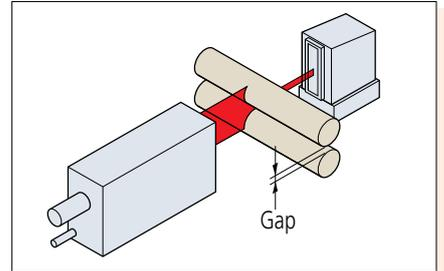
Measurement of tape width
