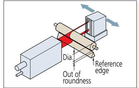
X- and Y-axis measurement of electric cables and fibers
