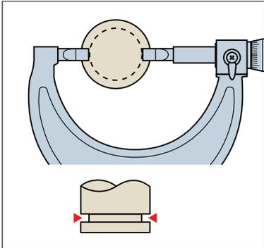
For diameter inside narrow groove measurement
