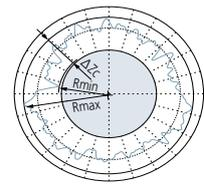
$\Delta Z_i = R_{max} - R_{min}$
