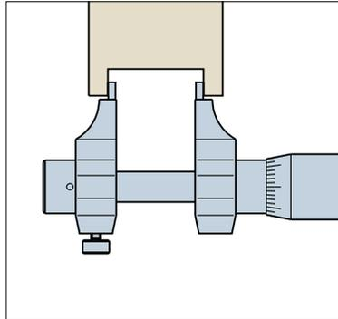
For small internal diameter, and groove width measurement
