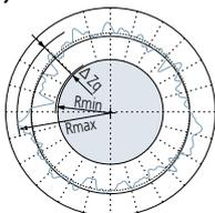
$\Delta Z_q = R_{max} - R_{min}$
