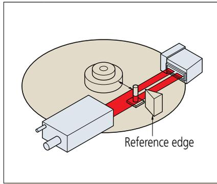
Measurement of gap between rollers
