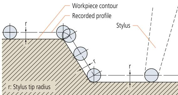
If a profile is read from the recorder through a template or scale, it is necessary to compensate for the stylus tip radius beforehand according to the applied measurement magnification.
