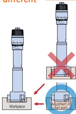
When you use the tip of the anvil for measurement, adjust the start point for using the tip of the anvil.
