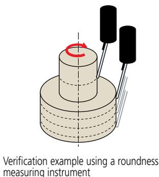
Specified direction: Radial direction Direction that intersects the datum axial straight line and is vertical to the datum axis line
