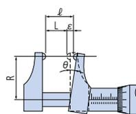
Abbe's principle states that "maximum accuracy is obtained when the scale and the measurement axes are common".
