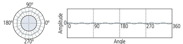
A 15 (or more) UPR condition is usually caused by tool chatter, machine vibration, coolant delivery effects, material non-homogeneity, etc., and is generally more important to the function than to the fit of a workpiece.
