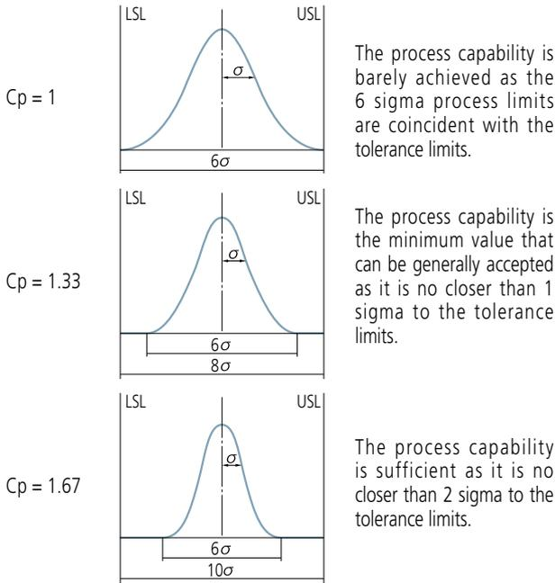
Note that Cp only represents the relationship between the tolerance limits and the process dispersion and does not consider the position of the process mean.
