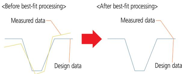
The best-fit processing algorithm searches for deviations between both sets of data and derives a coordinate system in which the sum of squares of the deviations is a minimum when the measured data is overlaid on the design data.
