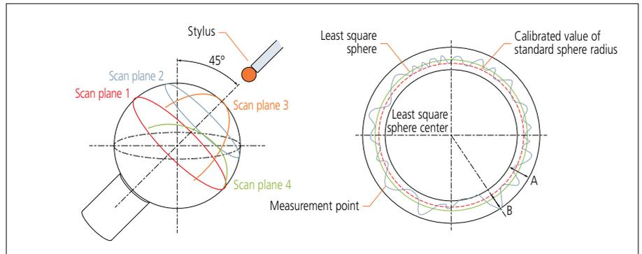
Figure 3 Target measurement planes for the maximum permissible scanning probing error and its evaluation concept
