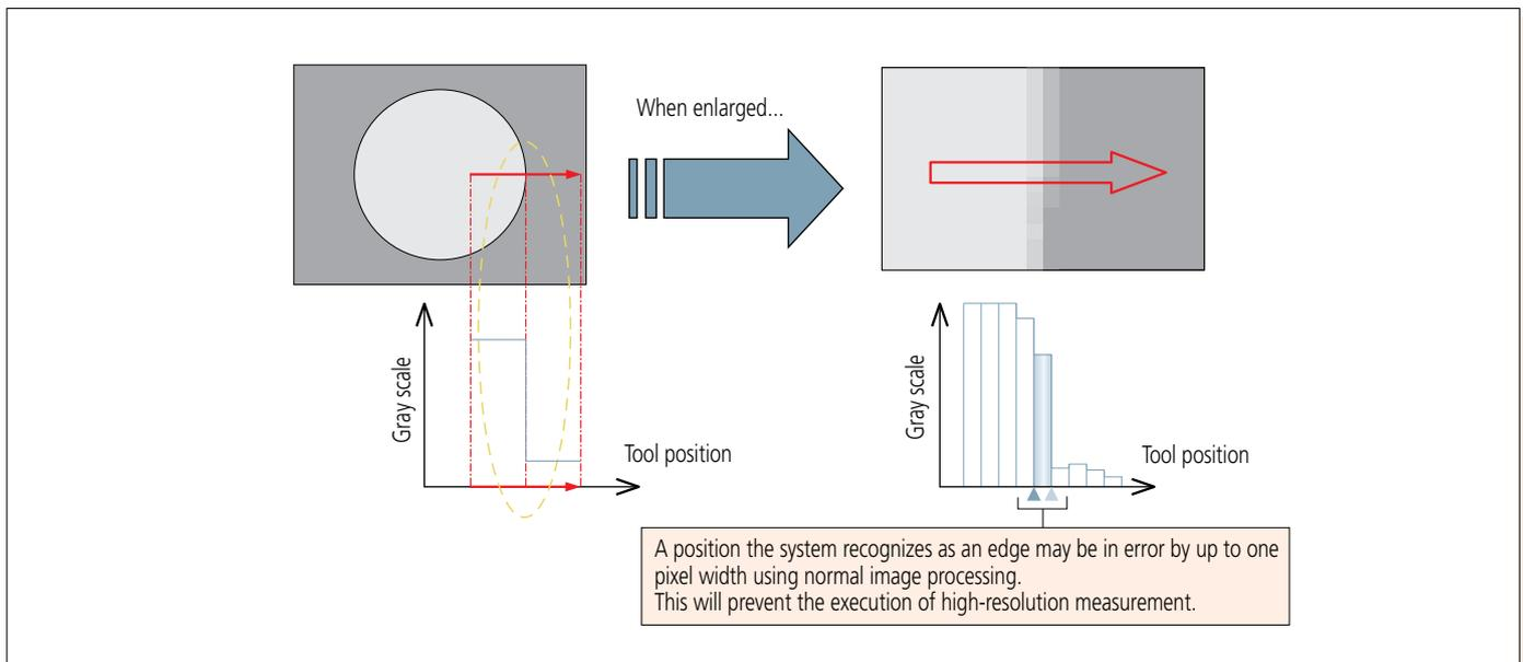
To increase the accuracy in edge detection, sub-pixel image processing is used. An edge is detected by determining interpolation curve from adjacent pixel data as shown below. As a result, it allows measurement with a resolution higher than 1 pixel.
