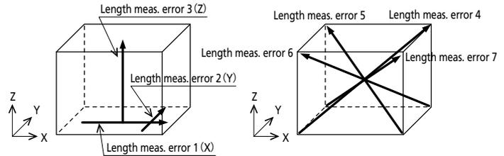
Figure 1 Measuring directions to obtain length measurement error
