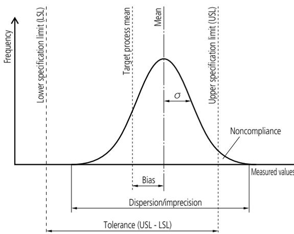
**Specific examples of a process capability index (Cp) (bilateral tolerance)**
