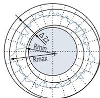
$\Delta Z_z = R_{max} - R_{min}$
