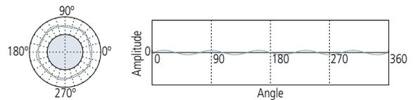
A 2 UPR condition may indicate: (1) insufficient leveling adjustment on the measuring instrument; (2) circular runout due to incorrect mounting of the workpiece on the machine tool that created its shape; (3) the form of the workpiece is elliptical by design as in, for example, an IC-engine piston.
