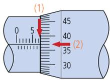
(1) Sleeve scale reading 7 mm
