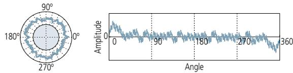
A 1 UPR condition indicates eccentricity of the workpiece relative to the rotational axis of the measuring instrument. The amplitude of undulation components depends on the leveling adjustment.
