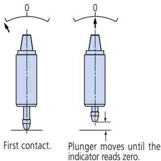
First contact. Plunger moves until the indicator reads zero.
