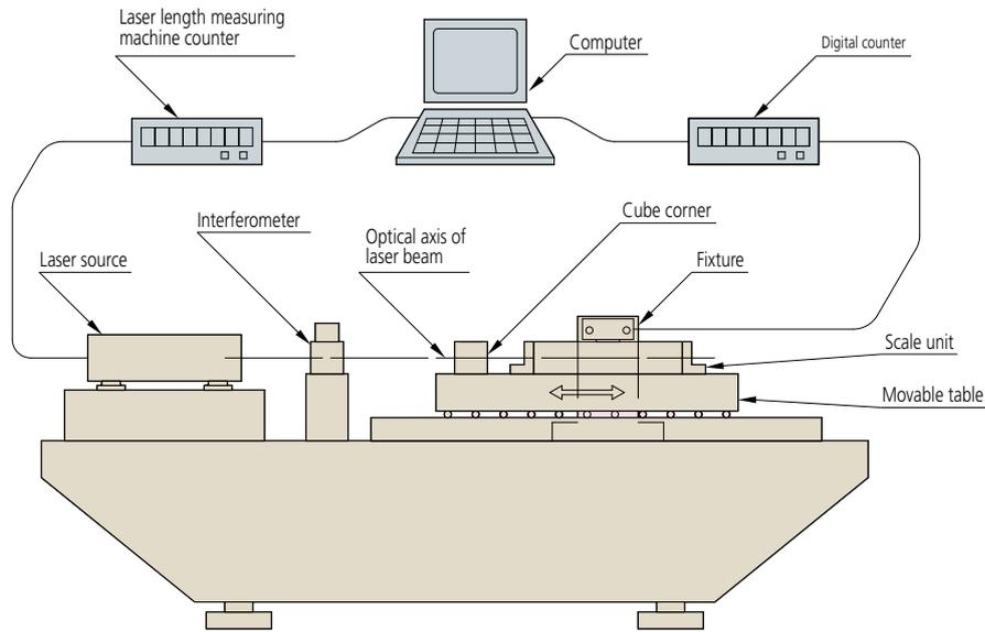
The accuracy of the scale at each point is defined in terms of an error value that is calculated using the following formula:
