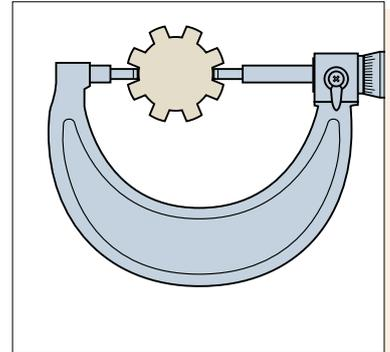
For splined shaft diameter measurement
