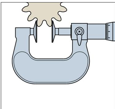
For root tangent measurement on spur gears and helical gears.
