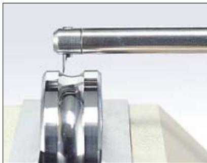
Inner/outer ring contour of a bearing
