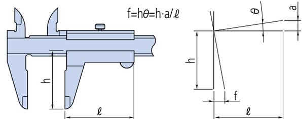
Example: Assume that the error slope of the jaws due to tilt of the slider is 0.01mm in 50mm and the outside measuring jaws are 40mm deep, then the error (at the jaw tip) is calculated as  $(40/50) \times 0.01 \text{ mm} = 0.008 \text{ mm}$ .
