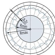
$\Delta Z_c = R_{max} - R_{min}$
