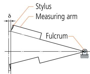
$\delta$ : Unwanted displacement in X to be compensated
