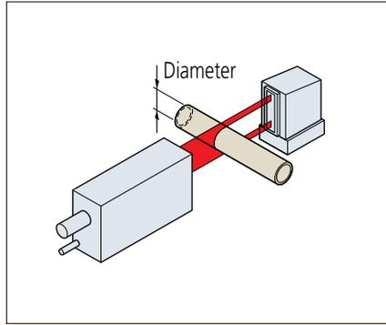
Measurement of outer diameter and roundness of cylinder
