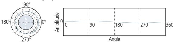
A 5 to 15 UPR condition often indicates unbalance factors in the machining method or processes used to produce the workpiece.
