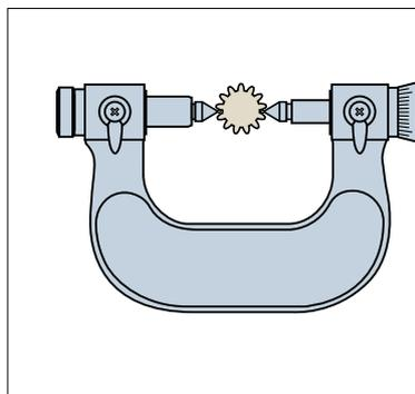
Measurement of gear over-pin diameter
