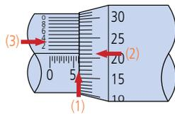
(1) Sleeve scale reading 6 mm
