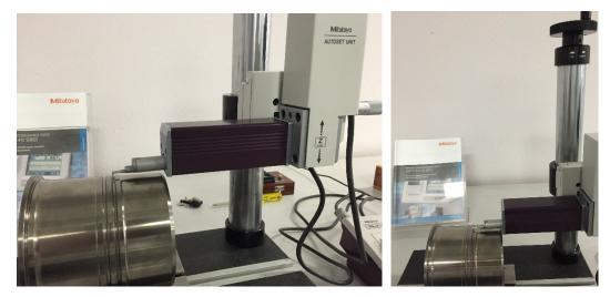
Auto-set unit, tilting adjustment unit, X-axis adjustment unit,
