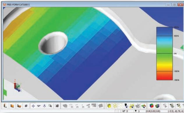
Surface deviation can be displayed as spherical points or as a gradient surface. Cones can also be used to show what direction of the deviation.
