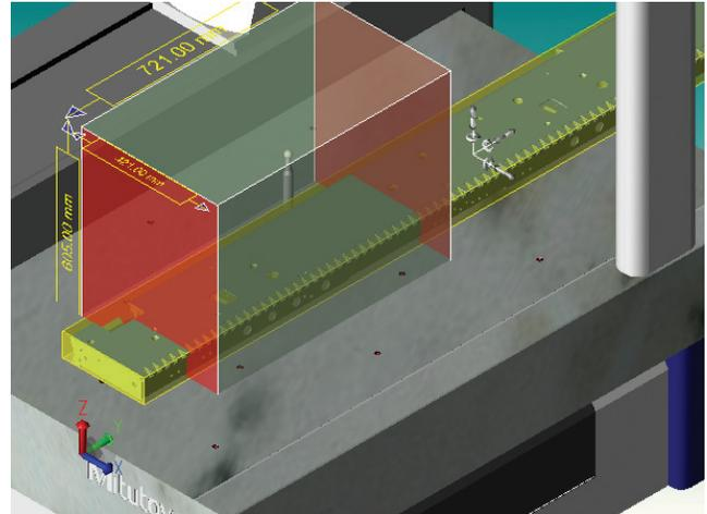
The CMM System Manager allows you create a virtual representation of your CMM for simulation. New Mitutoyo models or legacy models such as FN series and BHN series machines can be selected based on machine stroke. If you have multiple machines they can also be added for simulation or part placement purposes. CAD models can be placed and compared to the true working volume of the machine and indexing probe swivel access.
