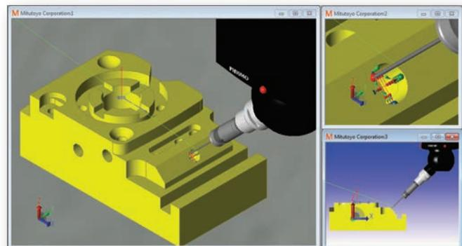
CAT1000P eliminates the time consuming task of data input from paper prints allowing your CMM to work in a paperless environment or by MBD (Model Based Definition).
