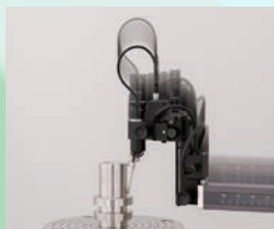
Spiral-mode cylinder measurement
