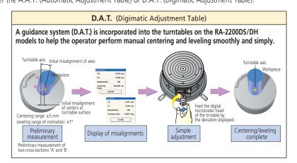
Centering and leveling using an A.A.T. or D.A.T.\* can be integrated in the measurement procedure (part program). This can prevent mistakes such as forgetting to center and level during measurement and is intended to standardize measuring work through part-program measurement.
