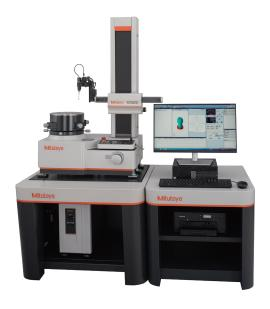
The photo shows RA-2200 +vibration isolator with side table.
