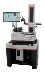
The photo shows RA-2200 + vibration isolator with monitor arm.
