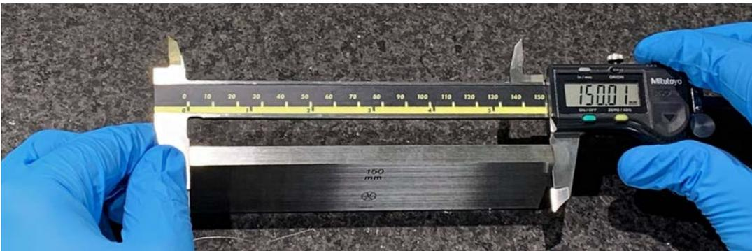
*Caliper calibration using gage blocks*
