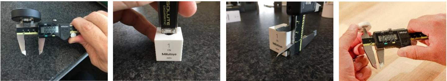
The internal measuring faces on many styles of calipers use crossed knife-edges. Due to the thickness of the faces and the clearance between them, additional errors can occur when measuring small internal diameters. For calipers that utilize cross knife-edge measuring faces, ASME B89.1.14 requires an additional test using a 0.2 in (5 mm) diameter ring gage for all calipers with measuring ranges up to 12 in (300 mm).
