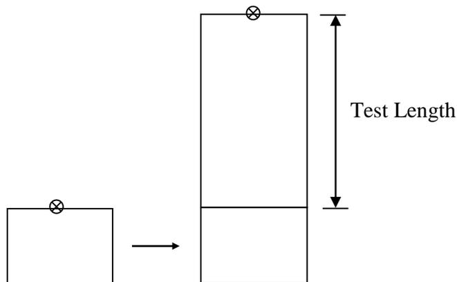
Figure 5. Example test of  $E_{UZ}$  using one gage block stacked onto another one which is used as the reference point.
