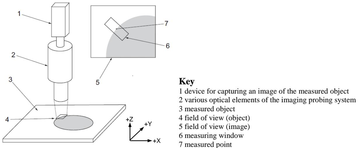
Figure 2. Example imaging probing system
