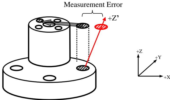
Figure 6. Measurement error associated with a squareness error in the XZ-plane. The  $Z'$  axis represents a possible error motion in an actual Z-axis, which results in measurement errors in two-dimensional measurements, as shown.
