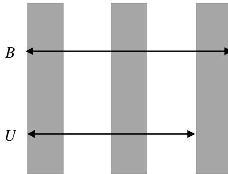
Figure 3. Many artifacts, e.g. a linescale, allow both unidirectional measurements (U) and bidirectional measurements (B). The artifact must be calibrated for the desired use.
