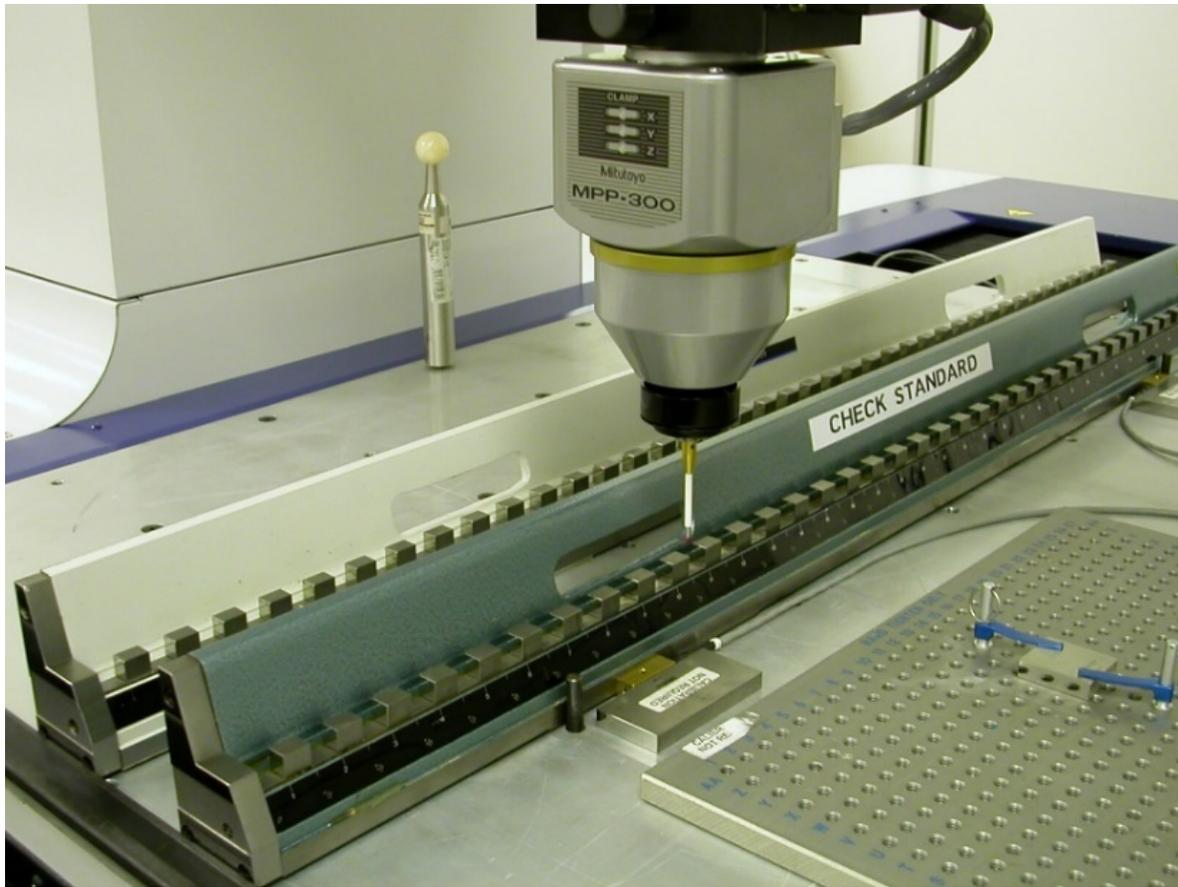
*A Mitutoyo Check Master being calibrated on a Mitutoyo Legex 910 CMM in the Mitutoyo America Calibration Laboratory. In the calibration of the Check Master, the purpose of calibration is to measure and report a calibrated length for each step of the gauge. There is no conformity assessment, as the Check Master is not typically used in that manner.*
