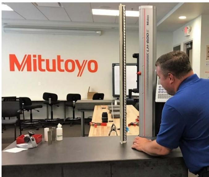
*Learning proper calibration technique for the Mitutoyo LH-600 linear height gauge in the Mitutoyo America training laboratory.*
