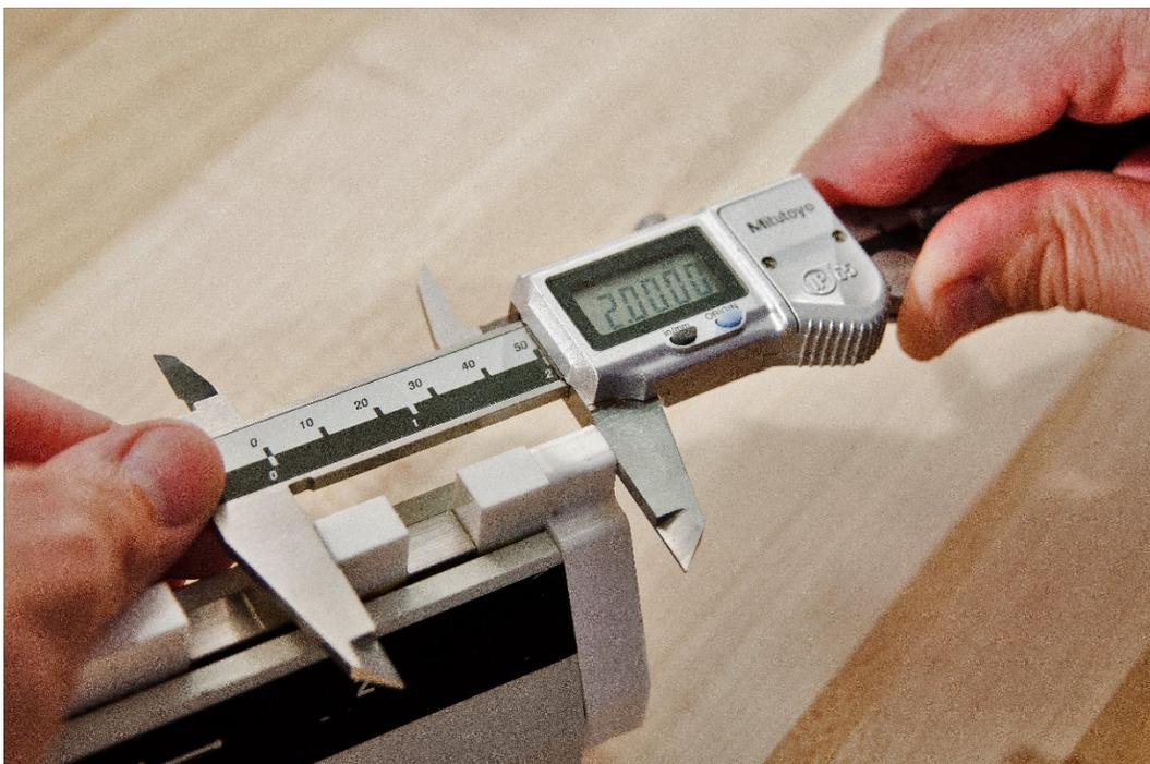
*Testing the partial surface contact error,  $E_{MPE}$ , with a caliper checker.*
