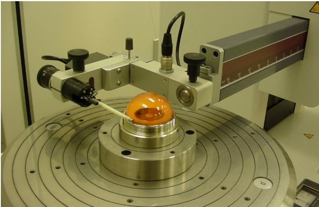
*Using a reversal method to measure roundness to 5 nanometers ( $0.2 \mu\text{in}$ ) in the Mitutoyo America Calibration Laboratory. Mitutoyo built a premier calibration facility to provide the support needed by Mitutoyo field service for the calibration of customer's measuring instruments.*
