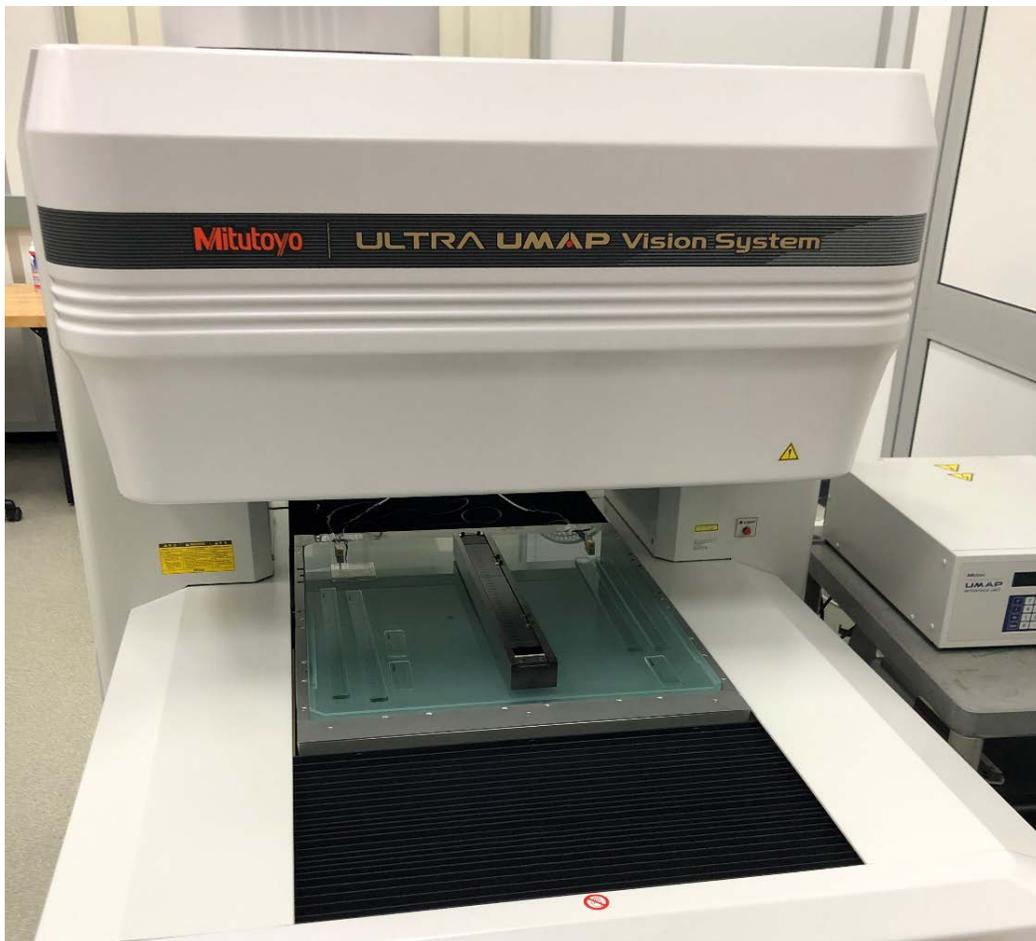
*The Mitutoyo QV Ultra vision system is used for high accuracy calibration of 1D and 2D glass artifacts in the Mitutoyo America Calibration Laboratory. The measurement uncertainty is as low as  $0.25\ \mu\text{m}$  ( $10\ \mu\text{in}$ ).*
