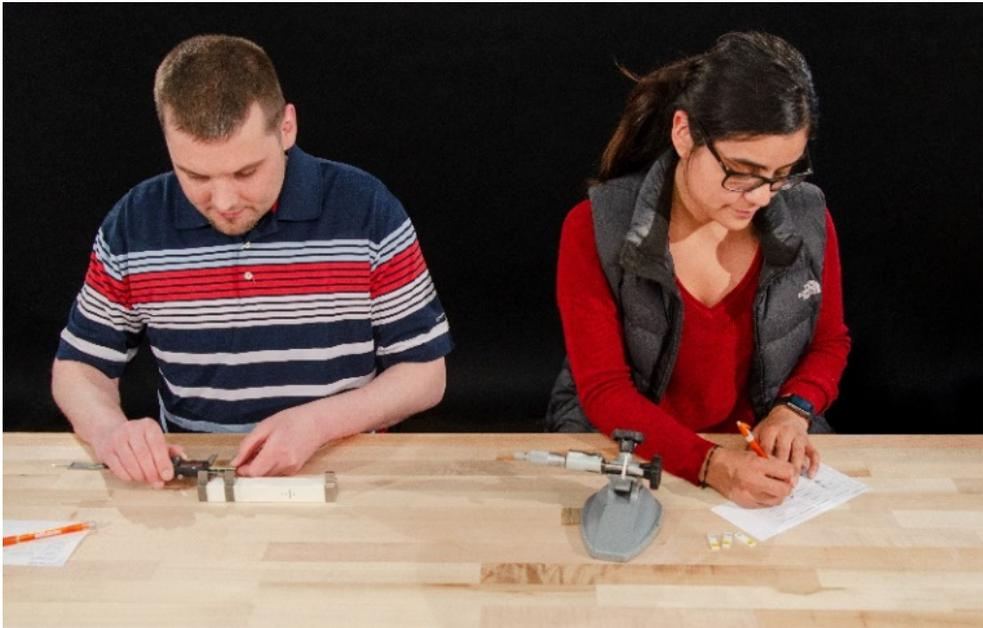
*Mitutoyo America offers a certification program in dimensional calibration that combines written theory tests plus hands-on skills performance tests. Shown here are participants testing their skills in micrometer and caliper calibration*
