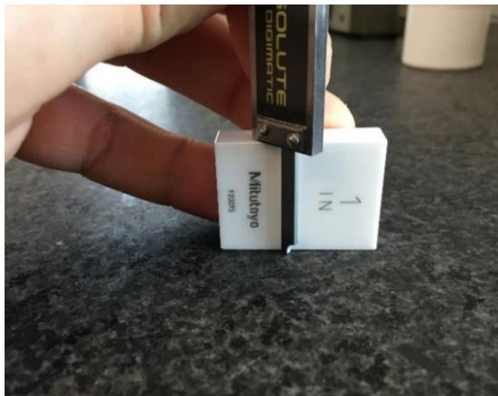
*A caliper is a hand-held, manually operated, measuring instrument. The accuracy specifications need to be valid for a user of sufficient skill and the caliper needs to be tested under that condition. Variation from the user is expected and is part of what is being tested. Variation from the user is not also a contributor to the test uncertainty.*
