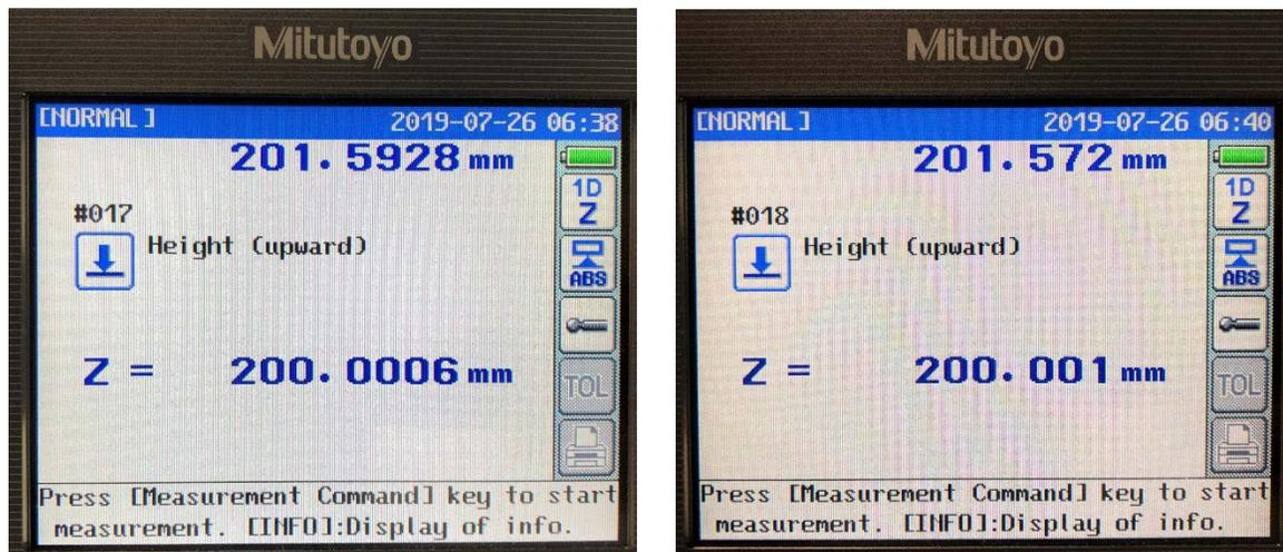
The Mitutoyo LH-600 has resolution that is selectable by the user of the measuring instrument. Changing the resolution of the LH-600 may change the measured value. Using the example measured values shown earlier in this chapter, the impact of changing the resolution is shown in the tables below.
