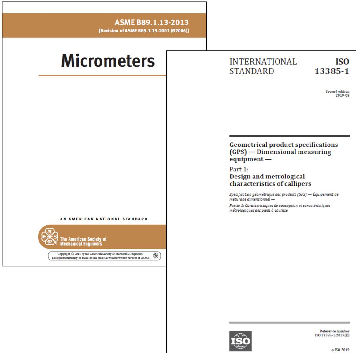
*The American national micrometer standard, ASME B89.1.13-2013, and the international caliper standard, ISO 13385-1:2019, were two of the first standards to specifically implement test uncertainty concepts.*
