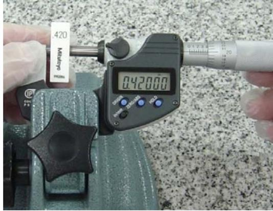
*Small dimensional measuring instruments like micrometers and calipers have rated operating conditions defined at 20 °C. In these situations, there will always be uncertainty due to temperature in the calibration. The material of the micrometer or caliper, the specific unit under test (UUT), needs to be considered in the uncertainty evaluation.*
