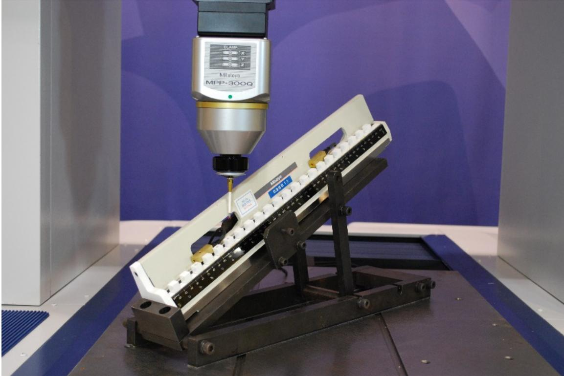
*ISO 10360-2:2009 requires three-dimensional, volumetric, testing. There may be many different calibration methods in practice for CMMs, but there is only one method that is standardized across all national and international standards. In the U.S., ASME B89.4.10360.2-2008 has the same general test methods as ISO 10360-2:2009.*
