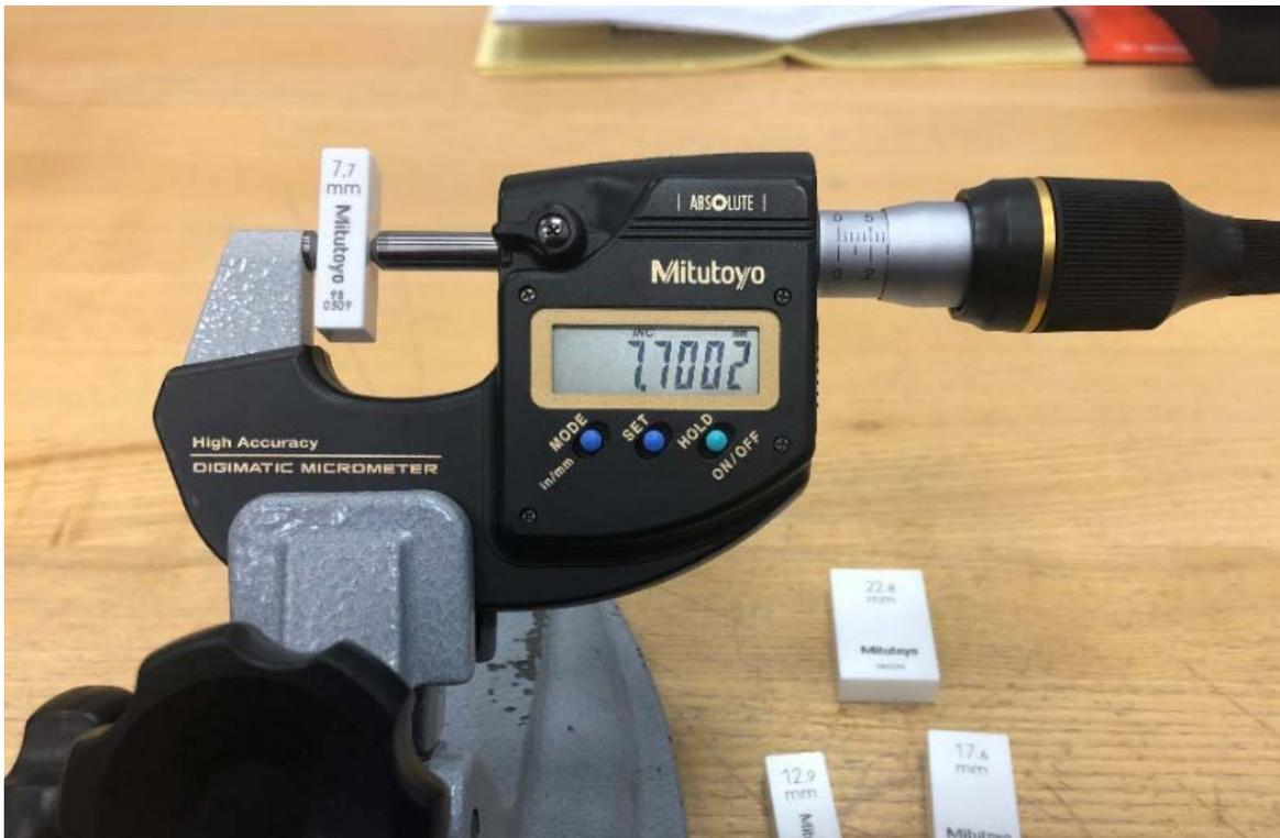
*Calibration of a high accuracy outside micrometer using gauge blocks. The resolution is 0.1  $\mu\text{m}$  compared to 1  $\mu\text{m}$  for a typical micrometer. The improved resolution helps the micrometer achieve an improved accuracy, but the resolution has no impact on the uncertainty of the test values in calibration.*
