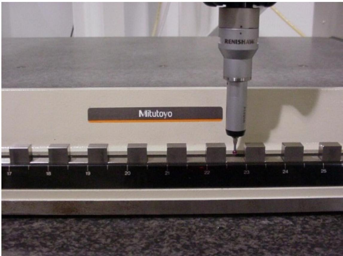
*When testing a manual CMM, the location of the measured point on the reference standard – in this case a Mitutoyo Check Master – will be less accurate. In this case, there is additional test uncertainty, associated with the flatness and parallelism of the measuring faces, due to this contribution from the specific unit under test (UUT).*
