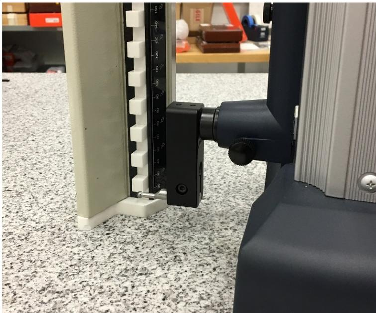
*Testing a Mitutoyo LH-600 Linear Height Gauge with a step gauge (a Mitutoyo Check Master).*
