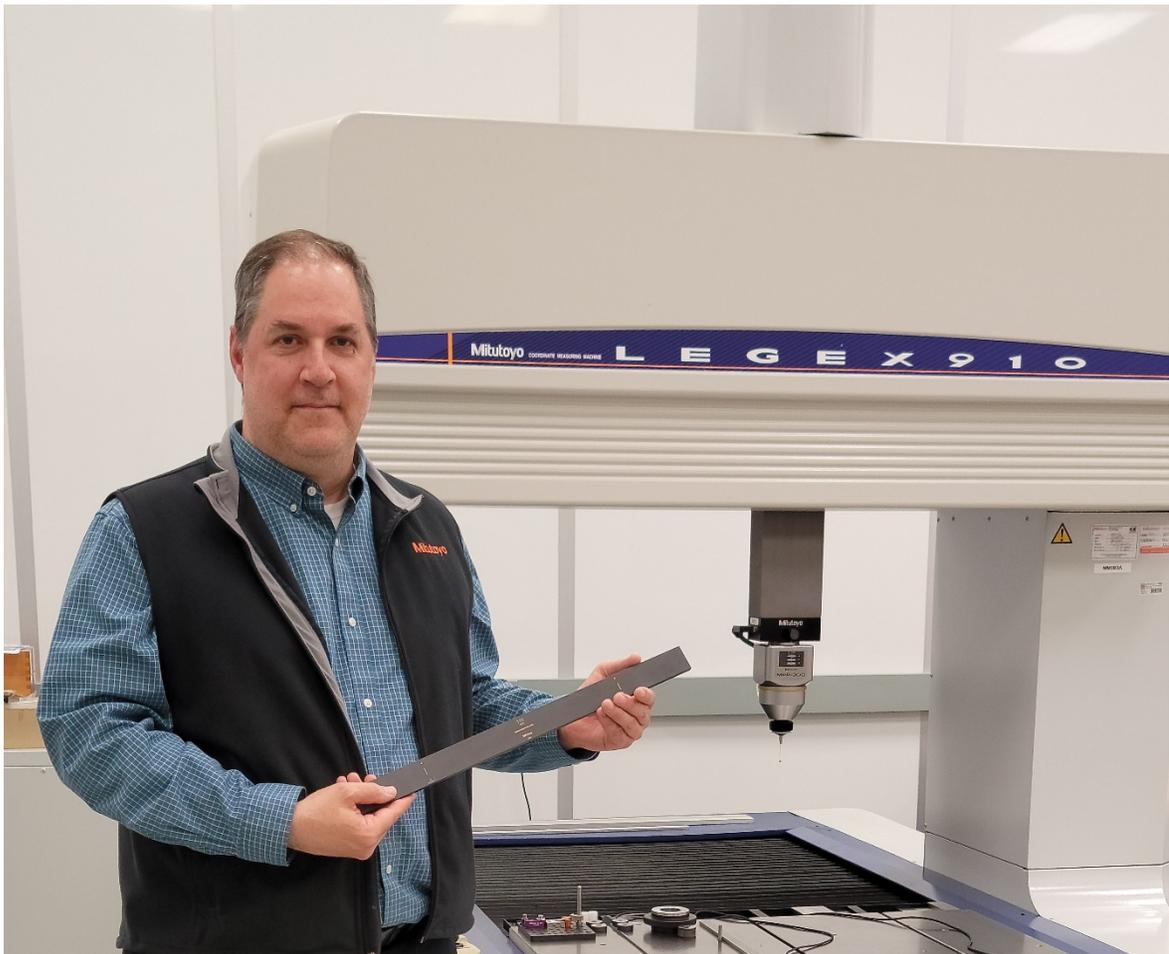
*The author in the Mitutoyo America Calibration Laboratory by his favorite ultra-high accuracy Mitutoyo Legex coordinate measuring machine holding the ultimate length standard – a Mitutoyo Zero CERA gauge block.*
