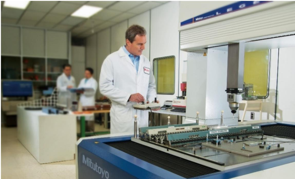
*The reference standard used to calibrate the Mitutoyo LH-600 Linear Height Gauge is a Mitutoyo step gauge called the Check Master. In the Mitutoyo America Calibration Laboratory, an ultra-high accuracy CMM, the Mitutoyo Legex 910, is used to calibrate Check Masters and other length standards with a measurement uncertainty as low as  $0.25\ \mu\text{m}$  ( $10\ \mu\text{in}$ ).*
