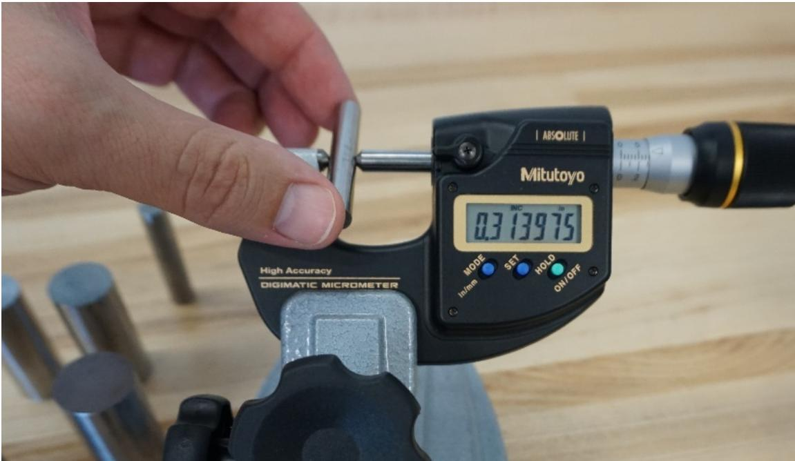
*Calibrating pin gauges with a laser scanning micrometer or high accuracy micrometer can achieve measurement uncertainty around  $0.5 \mu\text{m}$  ( $20 \mu\text{in}$ ).*
