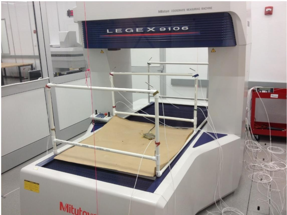
*Testing the temperature within the measuring volume of a high accuracy CMM at Mitutoyo America.*
