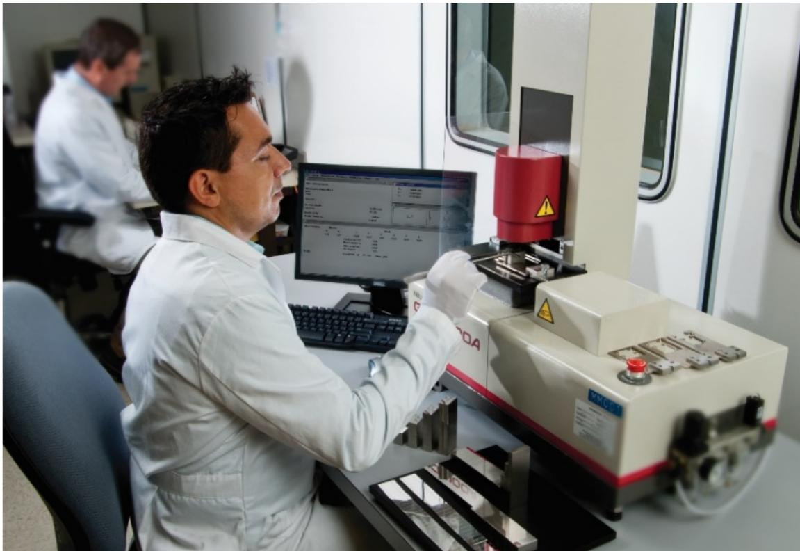
*Calibrating one of the over 50,000 gauge blocks that come through the Mitutoyo America Calibration Laboratory every year. Mitutoyo America calibrates all types and makes of gauge blocks and supports many of the other calibration laboratories in the US by calibrating their master gauge blocks. The gauge block comparator shown is the automatic gauge block comparator Mitutoyo GBCD-100A.*
