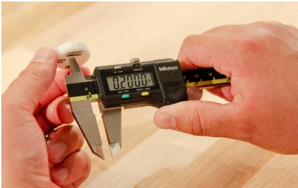
*The American standard for calipers, ASME B89.1.14-2018, requires testing the inside measuring function of certain styles of calipers using a ring gauge with a nominal size of 0.2 inch (5 mm). A single reading at this test point, with no averaging of multiple readings, is required. This type of specificity in the test protocol is critical.*
