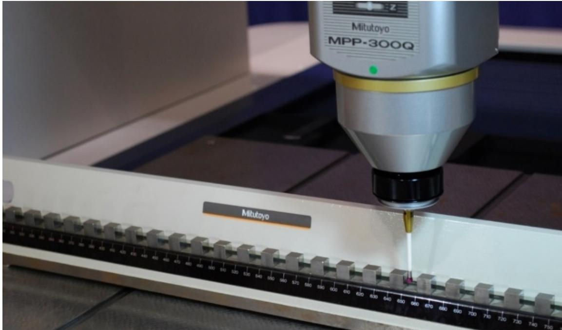
*Using a step gauge to test the conformity assessment of a CMM to  $E_{0,MPE}$  from ISO 10360-2:2009.*
