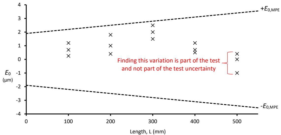
Example of testing a CMM in accordance with ISO 10360-2. The fifteen test values for one of the seven required measurement lines are shown in comparison to the tolerance of  $E_{0,MPE} = 1.9 + 3L/1000 \mu\text{m}$ . Three test values are reported at each of five lengths. The variation between the three values is part of the test and not a contributor to the test uncertainty.
