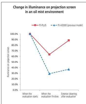
Adoption of the LED illumination source has eliminated the need for installing a cooling fan into the main unit of the measuring instrument and has drastically decreased the entry of oil mist, dust, etc. via the cooling fan into the instrument body.
