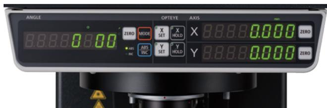
Since the digital counter (XY axes and angle) built into all models as standard uses a high-intensity LED and a large-character display, it secures high visibility unaffected by the environment. In addition to zero-setting and direction change, the data output of each counter value adopts the highly versatile RS-232C.
