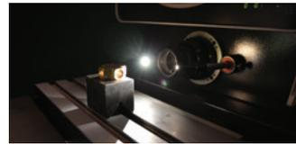
Includes Built-In Twin Fiber Optics to assist with the measure of surface features/defects.
