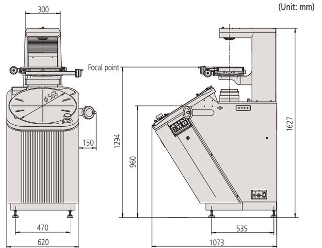
Note: To mount the counter (KA-212) and counter stand, approximately 300 mm space is required on the right-hand side of the main unit.
