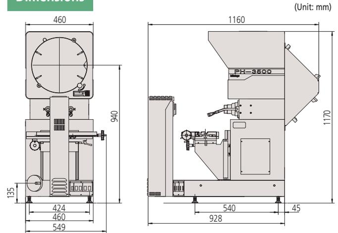
Note : To mount the optional counter (KA-212) and counter stand, approximately 300 mm space is required on the right-hand side of the main unit.
