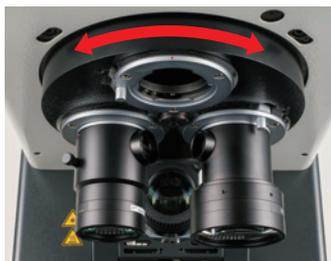
The turret of the PJ-H30 Series uses low-friction bearings that enable smooth and rapid rotary motion for changing magnification by bringing different projection lenses into the light path. The turret body uses bayonet mounts to aid quick attachment and detachment of lenses.
