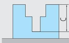
After measuring heights A and B, the height difference C between them can be shown in the lower row of the display.
