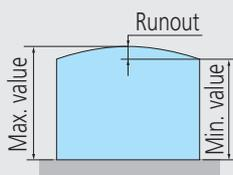
After scanning the surface, the runout will be shown in the display as (Max. value - Min. value)
