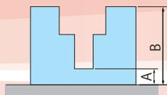
Height A and height B from the surface plate will be displayed.
