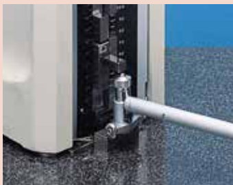
Bore gage zero-setting
