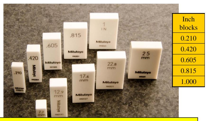
Both the US and the ISO standard recommend very specific test points for micrometers.
