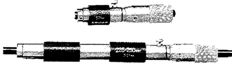
Fig. 3.1 Single rod type inside micrometer
