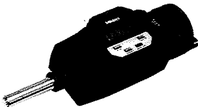
Fig. 5.11 Digimatic micrometer head
