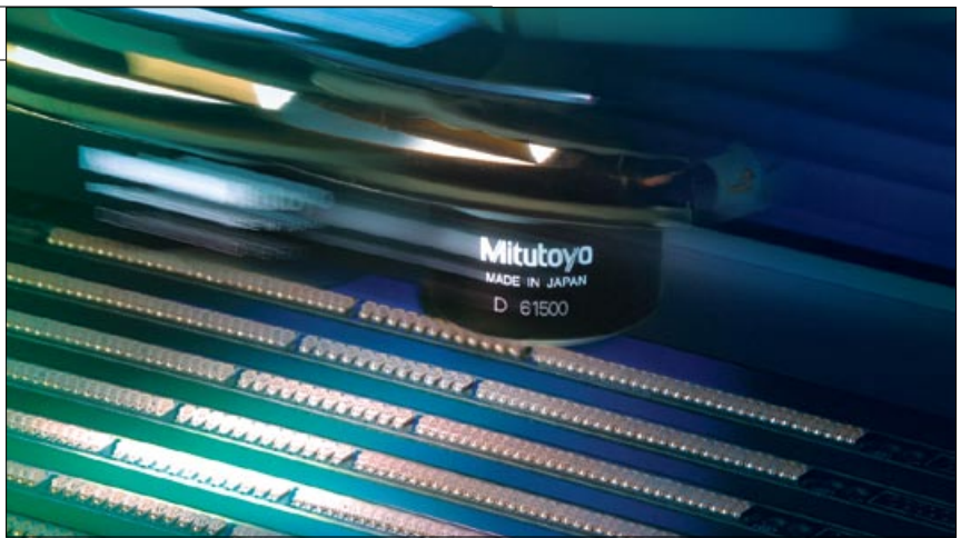
Vision dimensional metrology systems are an effective method for measurement and inspection for applications in which workpieces are delicate, easily deformed or very small. Source: Mitutoyo America Corp.
