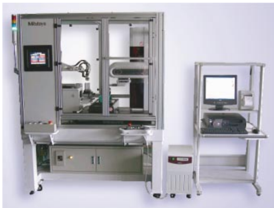
Example: Full automatic thin board surface roughness measuring machine
