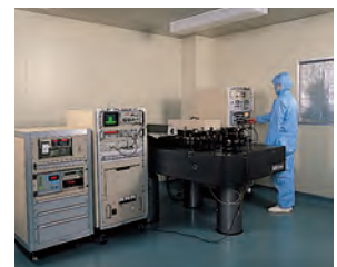
Iodine absorption stabilized He-Ne laser (633nm, for length standards)
