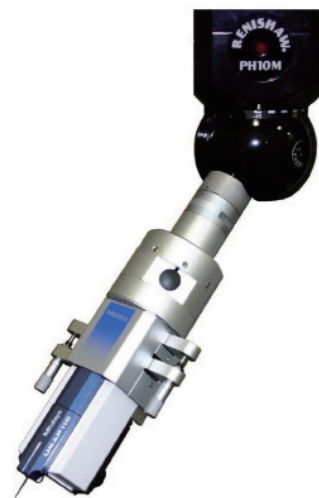
UMAP-CMM This head makes it possible to use an ultra-small diameter stylus (0.1- or 0.3-mm diameter). It can be installed on PH10MQ to measure the shape and dimensions of microfabricated products from multiple directions.
